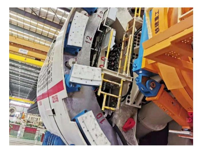
In urban rail transit, underground pipe gallery and tunnel construction, the shield machine is a key tunneling equipment. When the shield machine passes through complex geological structures, its shell and cutterhead are susceptible to strong friction and impact. In order to prevent damage to key structures and extend the service life of the equipment, a special protective device, a shield machine protective plate, must be installed.
