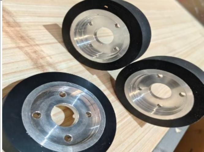
Three high-performance friction wheels are shown, arranged in a triangular pattern. Each wheel has a black rubber outer ring and a silver metal hub with four mounting holes. They are placed on a light-colored wooden surface. |
