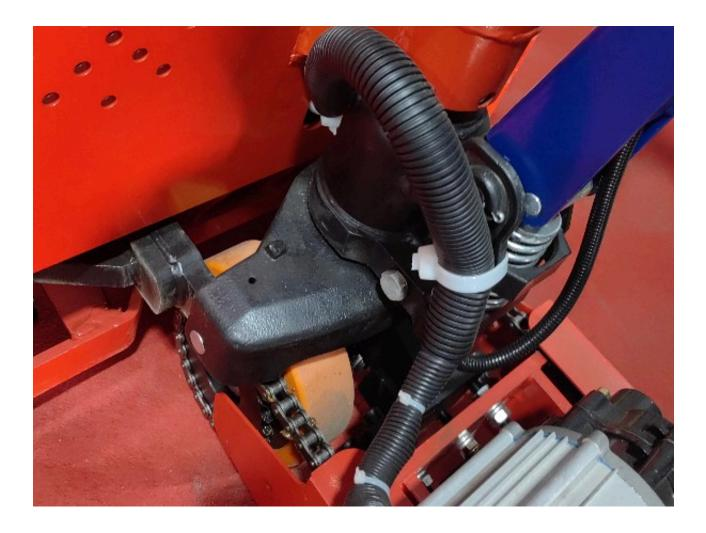
Load wheel (load-bearing core)
