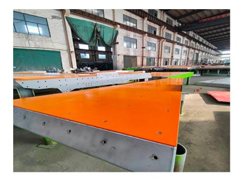
Features of cast anti-collision polyurethane plates
